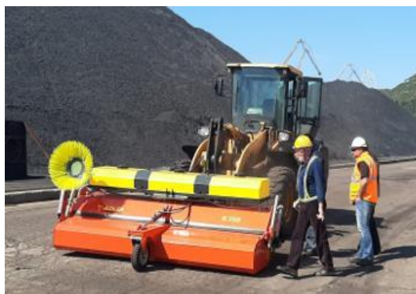
A road sweeper and a tractor-drawn tank for spraying the stored coal with a polymer emulsion are used daily.
